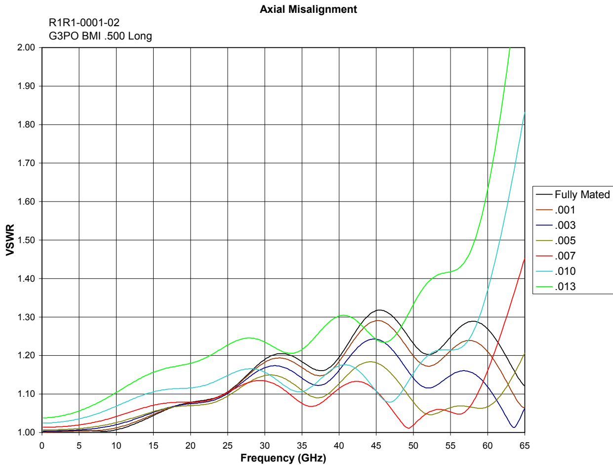
Figure 13 – G3PO Axial Misalignment Performance
