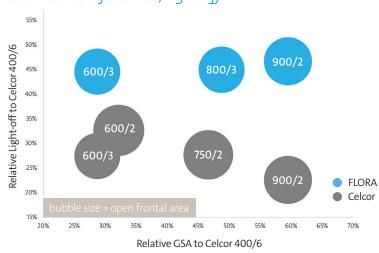
FLORA offers a clear upgrade path to reduce time to light-off and reduce emissions starting from any ultra-thin wall product.
