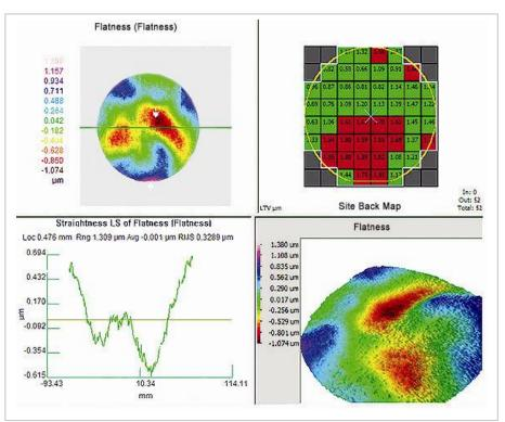
FlatMaster® wafer systems use a wide range of east to load wafer chuck to allow clamped or freestate measurements. Windows®-based software simultaneously tests wafers to multiple userdefinable global and site flatness parameters.
