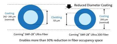
SMF-28 Ultra 200 fiber is the industry's first 200 micron fiber which provides low loss, meets and exceeds ITU-T G.652.D and ITU-T G.657.A1 industry standards, and features a 9.2 micron nominal mode field diameter (MFD) at 1310 nm for full backwards compatibility with legacy networks. Corning's CPC<sup>®</sup> coating technology provides the necessary optical and mechanical resilience required for outside plant cabling applications.
