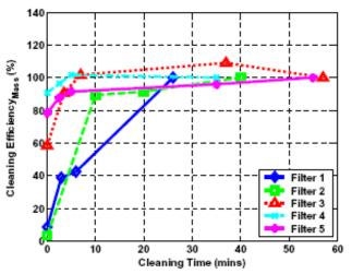
Figure 12. After about 20 minutes of cleaning with shop air (827 kPa pressure), most of the ash is removed from five different filters that were investigated. (50)
