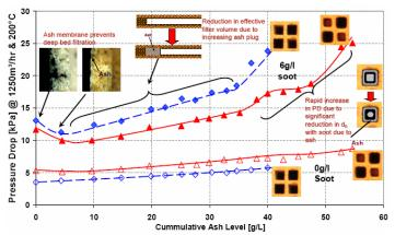
Figure 11. An initial ash layer prevents soot from penetrating the wall, resulting in lower back pressure upon soot loading than without ash. The triangles refer to an asymmetric cell geometry that provides more ash storage capacity. (49)
