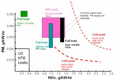
Figure 4. High load steady-state test results on HD research engines relative to the challenging US Not-to-Exceed in-use regulatory requirement.
