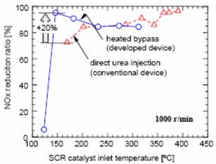
Figure 6. Decomposing urea at low exhaust temperatures using external heating provides a step improvement in SCR performance at T<200°C at 1000 rpm. (18)
