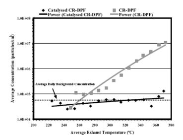
Figure 13. The average number of ultrafine particles increases with exhaust temperature primarily due to the formation of sulfuric acid aerosol nanoparticles (boxes). If the sulfate can be trapped, the ultrafine particle concentration in the exhaust is less than in ambient air. (51)
