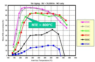
Figure 7. New zeolite SCR catalysts show impressive durability when occasionally exposed to temperatures of 800-850°C. (NTE refers to not-to-exceed temperature for design purposes.) reference 20.
