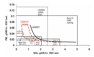
**Figure 2**. General comparison of on-road HDD standards in the US, Japan, and Europe. Estimated engine-out emissions for 2007 and 2010 (range) are shown. Steady-state cycle (3).
