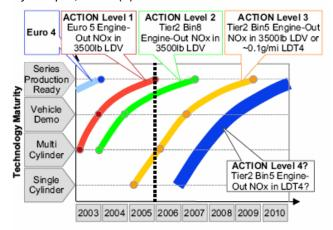
Figure 3. Light-duty diesel engine technology roadmap proposed by Cooper, et al. (6).
