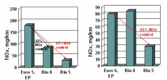
**Figure 1.** Euro 5 and Euro 6 light duty NOx regulatory proposals compared to the US. About 55-60% NOx control will be needed for a Euro 5 (2009) diesel to hit the
