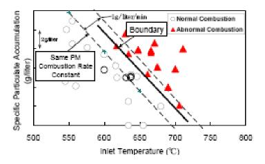
Figure 10. The threshold between normal and abnormal regenerations for cordierite filters depends on soot loading, DPF inlet temperature, and soot reactivity (dashed lines). Reference 38.
