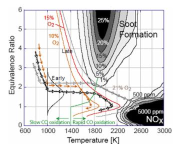
**Figure 4.** Principle of advanced combustion, wherein the flame temperature and equivalency ratio, , are kept away from NOx and PM formation regimes using injection timing and EGR (12).
