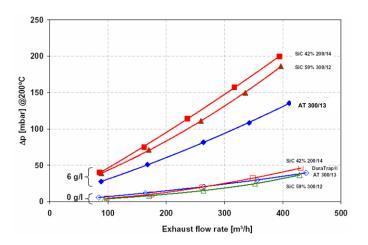
**Figure 15.** A new aluminum titanate filter that is now in series production has comparable unloaded back pressure as an SiC standard, but is 25% lower at 6 g/liter soot loading (57).
