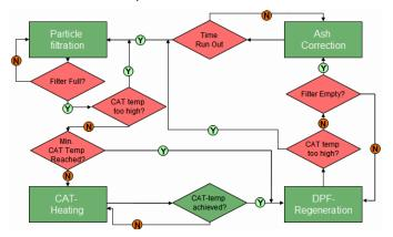
**Figure 12.** Example of LDD DPF regeneration plan. (45)
