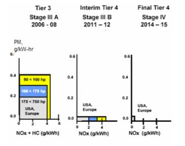
**Figure 3**. Future US and European non-road regulations for 50 to 750 hp engines (6).
