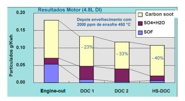
Figure 20. A new high sulfur DOC (HS-DOC) does ot form sulfates in 2000 ppm sulfur fuel, despite high temperatures (76).
