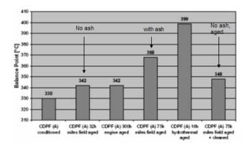
**Figure 16.** Ash can affect balance point temperature (65).
