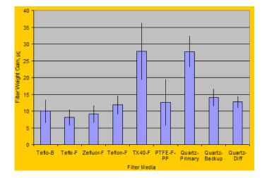
**Figure 18.** The choice of analytical filter can impact PM emissions results for systems using DPFs. Here two approved filters have 3.5X more emissions on them than other approved types (68).
