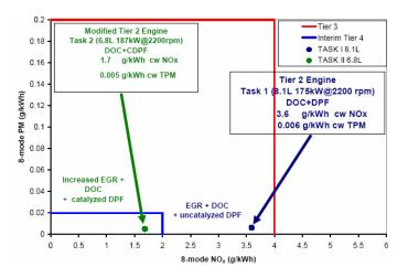
**Figure 23.** A interim Tier 4 (2011) non-road system, using high-pressure common rail fuel injection and cooled EGR to hit the NOx levels and a DPF to hit the PM levels. Fuel penalty is 3-5%. John Deere 6068H Tier 2 engine (83).
