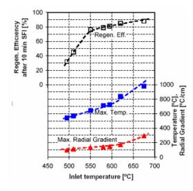
**Figure 14.** DPF inlet temperatures of >550C are needed to efficiently regenerate catalyzed cordierite filters with a 4 g/l soot loading. To further enhance regeneration, the inlet temperature can be increased later in the process (50).
