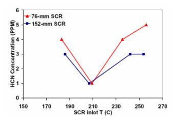
**Figure 6.** HCN formation from a reaction with  $NH_3$ , measured after an SCR system. HCN/NH<sub>3</sub> ratios are constant up to 6 ppm HCN (32).
