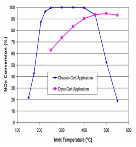
**Figure 7.** LNT efficiency for LDD (chassis certified) and HDD (dyno certified) applications (33). LT performance is critical for most LDD applications, whereas HT efficiency under high NOx fluxes is needed to meet HD NTE requirements. Hydrothermal aged 5 hours at 850C, 30,000/hr and 120,000/hr space velocities, respectively.
