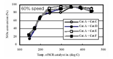
**Figure 5.** NOx removal efficiency curves for various SCR catalyst configurations (22). "Catalyst A" is an oxidation catalyst to promote the fast  $NO_2/NO/NH_3$  reaction. "Catalyst C" is vanadia-based, and the remaining catalysts are zeolite (25% smaller than the vanadia system).
