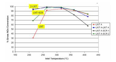
**Figure 9.** When an SCR is added to an LNT, system efficiencies go up (26).
