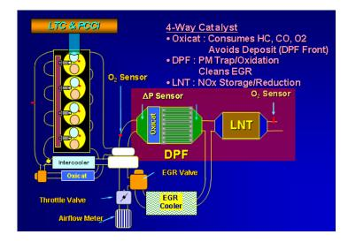
**Figure 22.** Example of an integrated emission control system for a mixed mode LDD engine. Converse to typical LDD architecture with traditional diesel combustion, the LNT is behind the DPF as LT NOx control is no longer a major issue (81).
