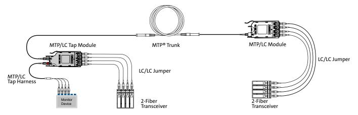
In the above scenario, the configuration B EDGE tap module is deployed as an integrated part of the structured cabling system to support serial duplex transmission. Within the system, the tap module functions like a normal Universal-wired module, while also sending the split signal to the MTP TAP port. This deployment eliminates the use of extra rack space and maximizes the channel reach by reducing the number of loss components in the system.
