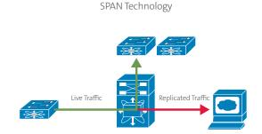
Active data extraction, typically called switch port analysis (SPAN) or port mirroring, uses an electronic device (usually a switch) to replicate, or mirror, the link's data and send it to a monitoring device.
