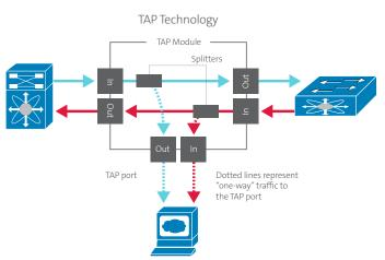
**Port tapping**, which is completely passive, extracts the data via a device that can split signals from both directions between its intended recipients as well as a monitoring device.
