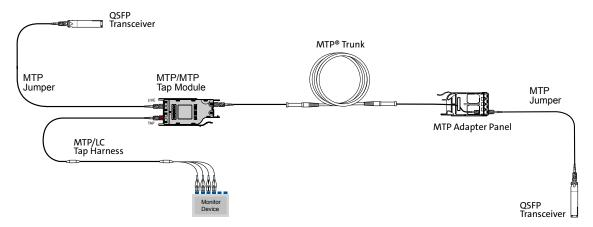
When migrating from duplex transmission to higher data rate via parallel transmission such as 40G, MTP equipment connectivity is required. The above scenario depicts the use of an EDGE8 Configuration C tap module for a parallel transmission system. A MTP jumper is used to interconnect the MTP parallel link equipment port to the MTP LIVE port in front of the tap module. When the monitoring equipment can receive a parallel input, a MTP/MTP tap harness is used to interconnect to the monitor device.
