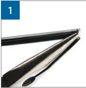
Figure 9. Advanced Stripping Process Starts With Commonly Used Hand Tools to Initiate Jacket Peel
