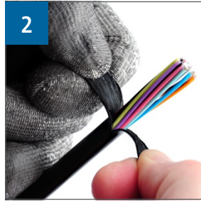
Figure 10. Cable Jacket Then Simply Pulled Apart to Required Stripping Length
