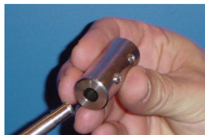
Figure 6. Slide larger opening on coupling collar over paddle shaft (Step 4).
